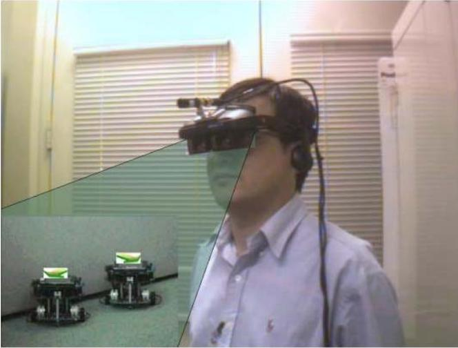
**Figure 6: Coded infrared signals are decoded into arrows for overlay onto a real scene. These are visible via the augmented reality head-mounted display system with camera.**
